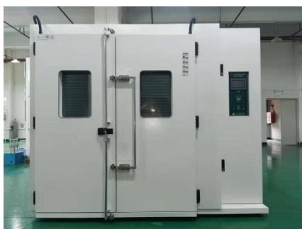
3.6 m3 constant temperature humidity laboratory
